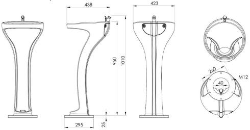
Fountain body: top ring Ø 423mm, base Ø 295mm Height of fountain body: 950mm, height of fitting: 60mm, total height: 1010mm above top edge of pavement Opening size of inspection flap: approx. 240mm x140mm Weight: approx. 17kg Material / surface:
